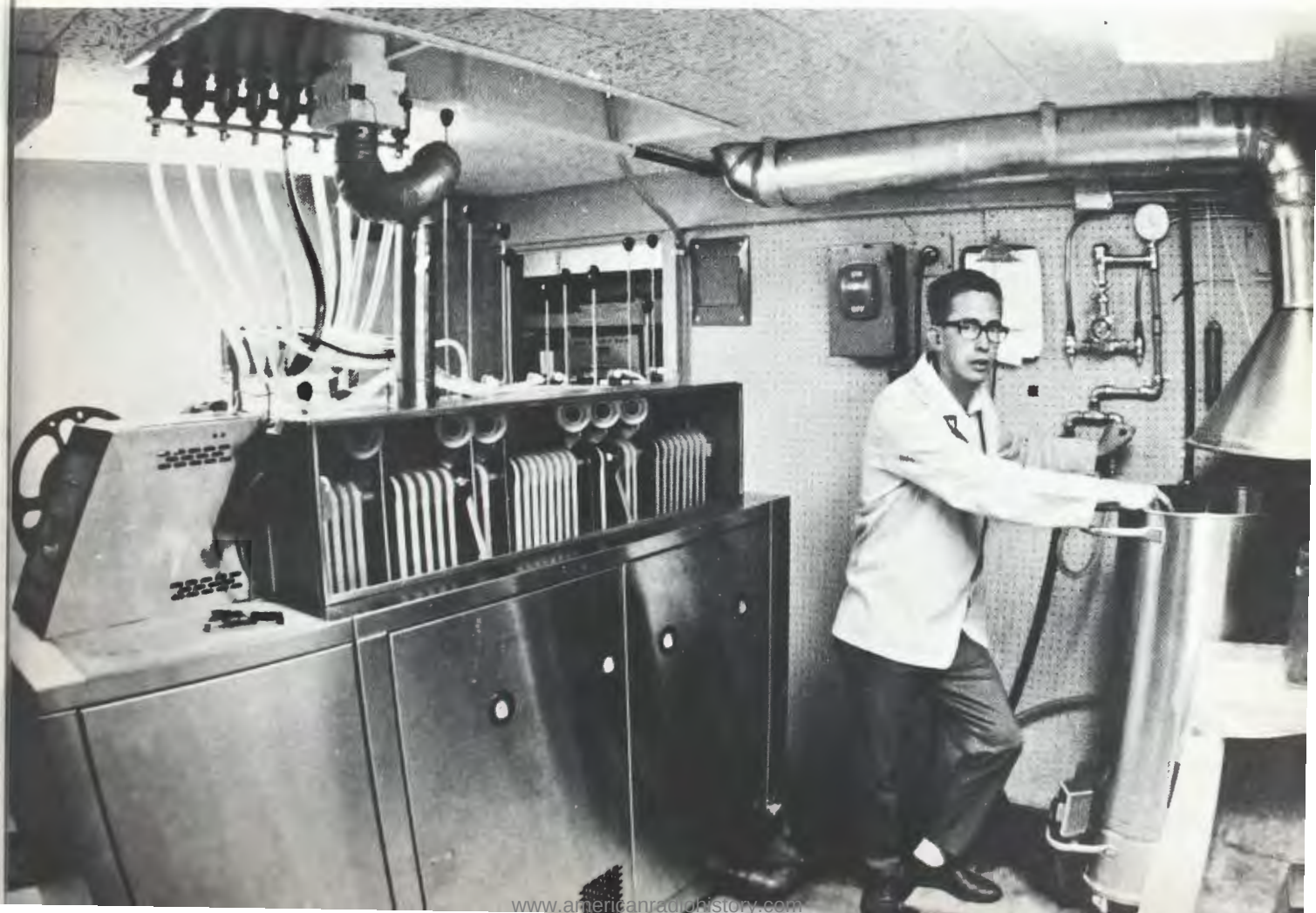
Fig. 1 KID-TV color processor installation with operator preparing to mix chemicals. Note cutout in ceiling to accommodate film transport rods. Replenishing lines and exhaust duct also run through the cutout.
